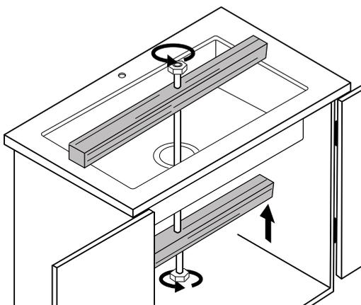
Clamp the sink and hold in place while adhesive cures. There are different methods, we suggest using a couple of pieces of wood with a threaded rod. Set one piece of wood under the sink and another over the countertop.
