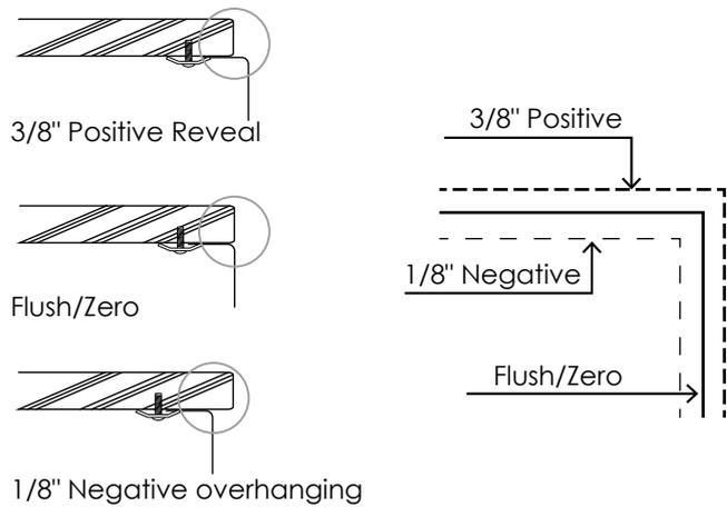
Use scissors to cut along the line of the paper template for you desired reveal type (Negative, Positive or Flush Reveal)
