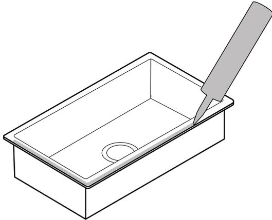
Clean sink flange and underside of cut-out area of countertop, making sure that the area is smooth and free of debris. Apply continuous bead of silicone caulk evenly on top of sink flange.
