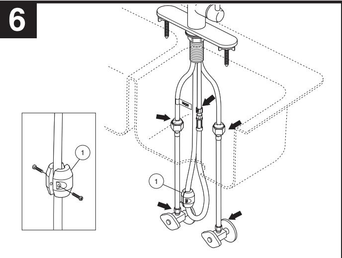
Attach the zinc weight (1) to the hose assembly in the approximate area shown. The weight should be on the upward swing of the hose, toward the spray head, to the mounting shank in order to provide proper pull to the hose. If further retraction is desired add a second weight. Make sure copper inlet tubes do not interfere with spray hose assembly. Hose assembly should pull freely through spout hub. Check all connections at arrows for leaks.
