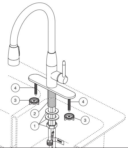
**Shut off water supplies.** Remove old faucet. Slide escutcheon and gasket (1) up over hose and tubes and underneath the faucet. Make sure the gasket is properly seated under the escutcheon, and place the faucet over the mounting holes.
