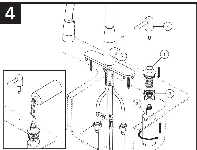
Snap the quick connect hose assembly (1) onto hose (2). Pull down moderately to ensure connection has been made. Spread the tubes (3) to desired position by grabbing near the top of the tubes. **WARNING:** Kinked tubes will void the warranty. Make connections to water lines (HOOK-UPS NOT PROVIDED). **Important:** When making connections be sure to use two wrenches when tightening. **Do not over tighten.**
