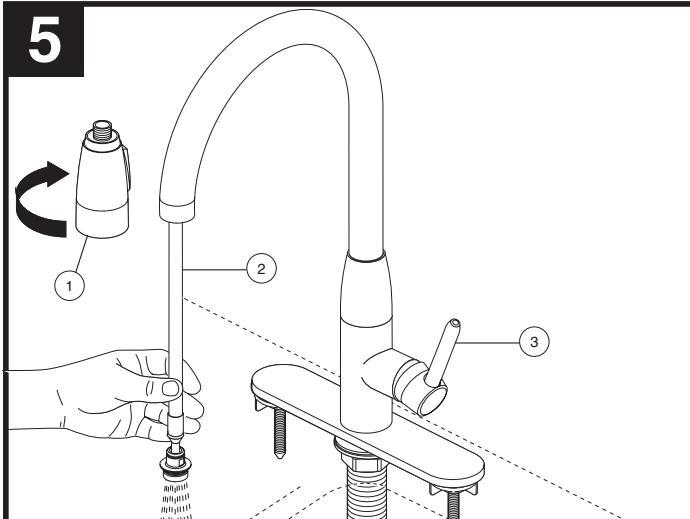
Remove sprayer assembly (1). Pull the hose assembly (2) out of the spout and be sure to hold the end of the hose down into the sink. Turn faucet handle (3) to the full on mixed position. Turn on hot and cold water supplies and flush water lines for one minute. Reinstall sprayer assembly.
