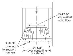
(Platform must be able to support cabinet load, weight of oven, and additional oven loads)
