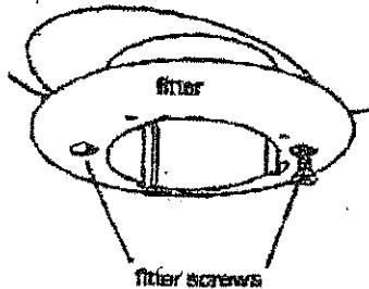
REMOVE GLOBE: slide filter to the side of the globe and lift out.
