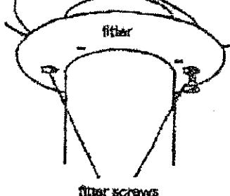
ATTACH GLOBE TO FITTER. Slide edge of globe between filter and one flange. Push other flange into globe. Center globe on filter. Tighten two filter screws to secure globe to filter.
