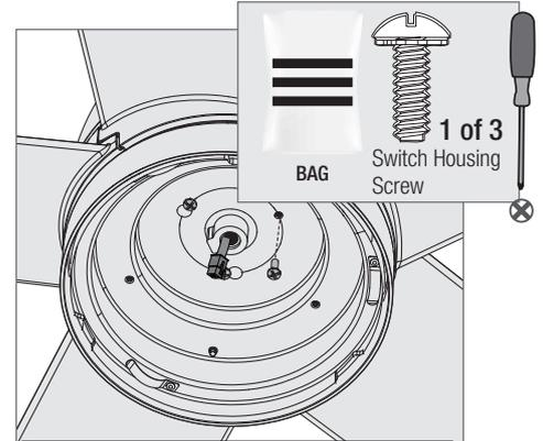
Insert the third screw found in the hardware bag, into place and then tighten all three screws.
