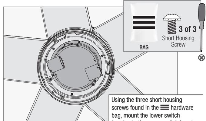
Using the three short housing screws found in the hardware bag, mount the lower switch housing to the upper switch housing.
