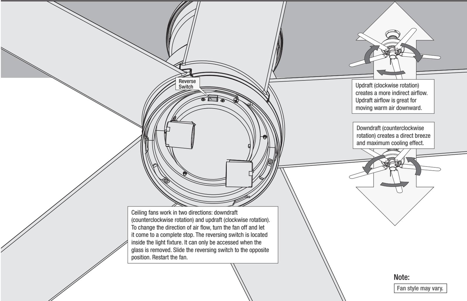
Ceiling fans work in two directions: downdraft (counterclockwise rotation) and updraft (clockwise rotation). To change the direction of air flow, turn the fan off and let it come to a complete stop. The reversing switch is located inside the light fixture. It can only be accessed when the glass is removed. Slide the reversing switch to the opposite position. Restart the fan.
