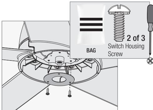
Partially install two switch housing screws, found in the hardware bag, through the gasket halfway into the motor housing as shown. It does not matter which two screw holes you choose.
