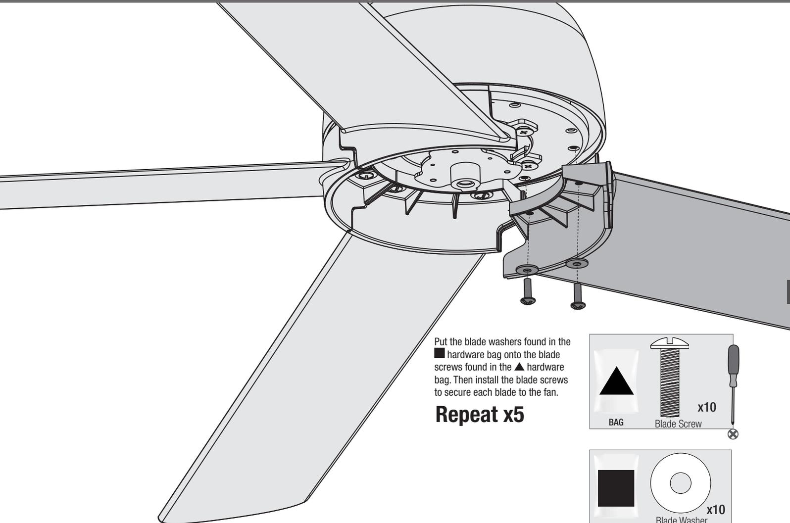
Put the blade washers found in the ■ hardware bag onto the blade screws found in the ▲ hardware bag. Then install the blade screws to secure each blade to the fan.
