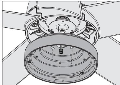
Feed the wire plug through the center hole of the uppers switch housing. Align the keyhole slots in the upper switch housing with the two screws you just installed. Lift the upper switch housing so that the keyhole slots engage the two screws, and twist counterclockwise to lock the upper switch housing into place.
