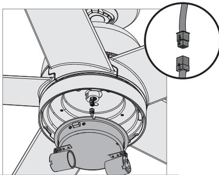
Lift the the lower switch housing and connect the plugs. Make sure to line up the colored markings on the connectors and that the connectors latch.
