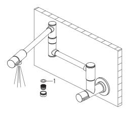
After the installation is complete, remove the aerator and housing by unscrewing it from the spout in a counterclockwise direction. Turn on the two handles to the right, turn on the water supply and allow water to run for at least one minute. This flushes away any debris that could cause damage to internal parts. Check for leaks. Reattach the aerator and housing. Do not lose the washer (1) in the aerator.
