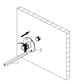
Install the seat (C) onto the finished wall. Screw the seat onto the supply piping and mark the locations for the support screws with a pencil (1).
