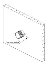
Install the supply piping so that the 1/2-14NPSM-2A threaded connection protrudes approximately 1/2-14NPSM-2A beyond the finished wall.
