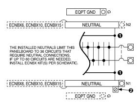
NEUTRAL BUS FOR PLUG-ON NEUTRAL CIRCUIT BREAKERS BOND WHEN REQ'D
