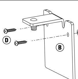
Align bracket [B] and attach with screws [D] (or use hardware suitable for your backsplash material).
