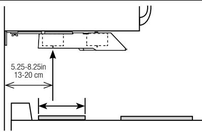
The center of the rear canister must be over the rear burner. If not, go to [www.STFS.com](http://www.STFS.com) to order an extension bracket kit.
