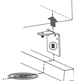
Slide wall bracket up to touch bottom of microwave or cabinet.
