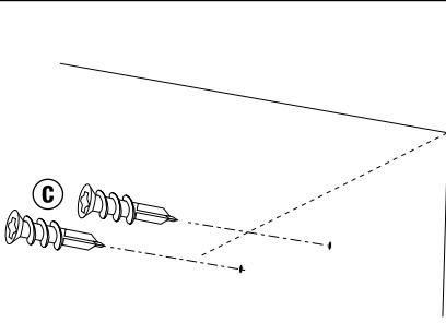
Tap anchors [C] into pilot holes. Hand tighten with #2 Phillips screwdriver (Use in drywall only.)
