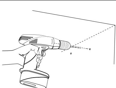
Drill 1/8" pilot holes in the marked locations. If wood stud is present behind drywall, proceed to Step 7.
