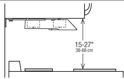
Must have 15-27" (38-68 cm) between surface of stove top and mounting point under microwave hood.
