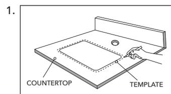
hole, so they must be large enough to fit the blade of a jig saw or keyhole saw.
