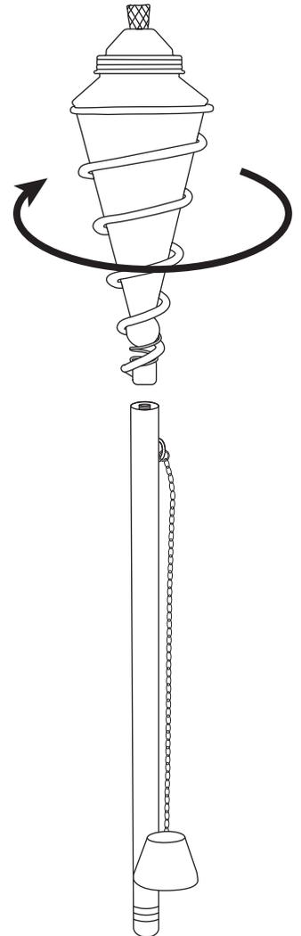
1. Connect the ring on the snuffer chain to the loop on the side of the Top Pole.
