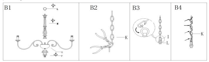
Step B1: Carefully thread post (M),drops (P) onto the fixture (O),then thread the loop (L) onto the post (M).
