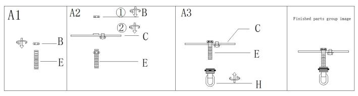
Step A1:Thread hex nut (B) onto the nipple (E)
