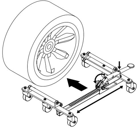
b. Move the Lever to the up position, then pump the Foot Pedal until the tire is just lifted off the ground.
