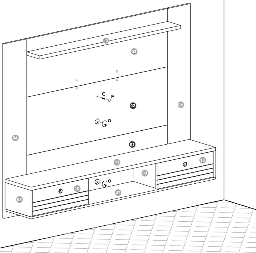
**IMPORTANT!** To remove the panel from the wall, to unscrew the security bolt (C) applied as in the STEP 8 and moving it upwards slightly so as to disengage the chamfered edges of the Bars (06) and (13) fixed behind the panel and on the wall. Before moving the panel, remove TV and other objects that are installed and ensure that the entire set is safe, preventing falls and damage to the panel and equipment.
