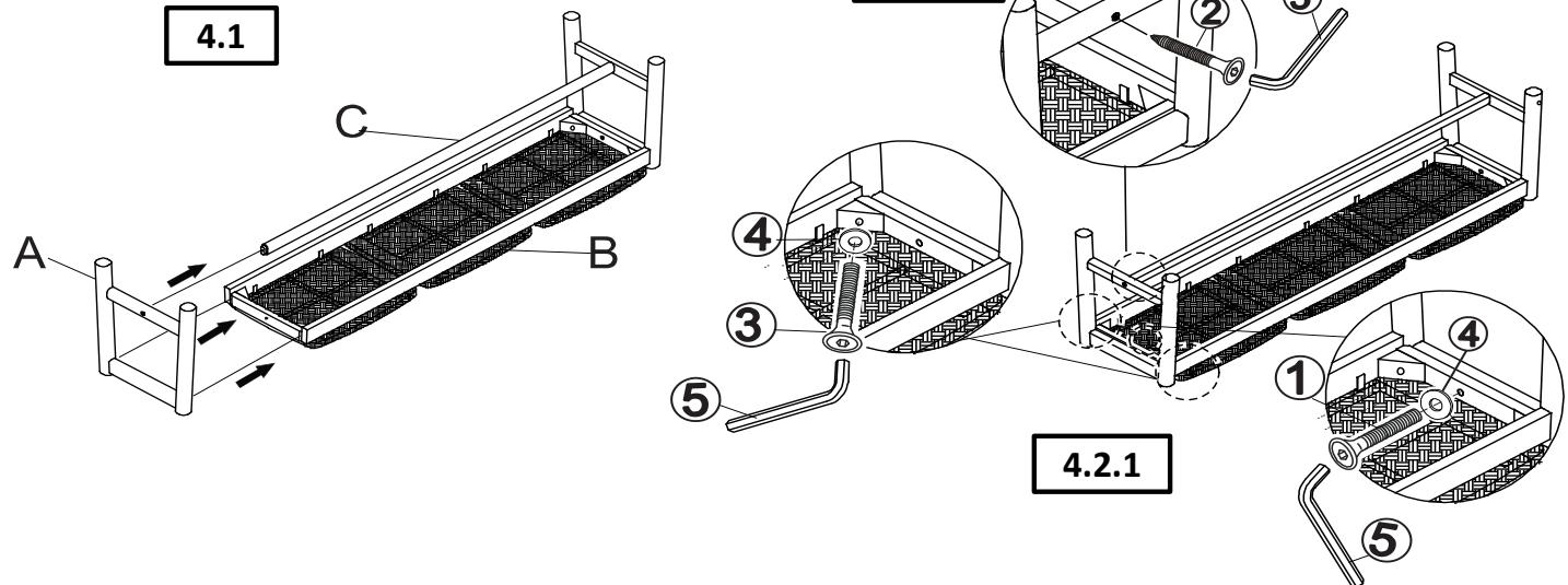
Repeat the same process to attach the remaining Leg Panel (A) to the Seat Panel (B) and Support Bar (C)
