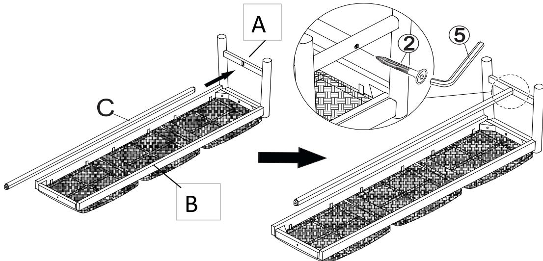
Affix the Support Bar (C) to the Leg Panels (A) using Screws (2) and the Allen Key (5).
