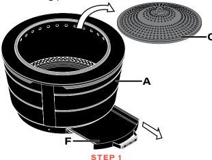
Remove the ash pan (F) and dome insert (C) from the Fire Pit (A) and set aside.
