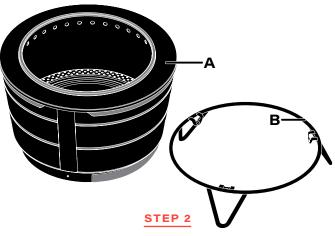
Separate the Fire Pit (A) from the foot ring (B) and place the foot ring on its feet.
