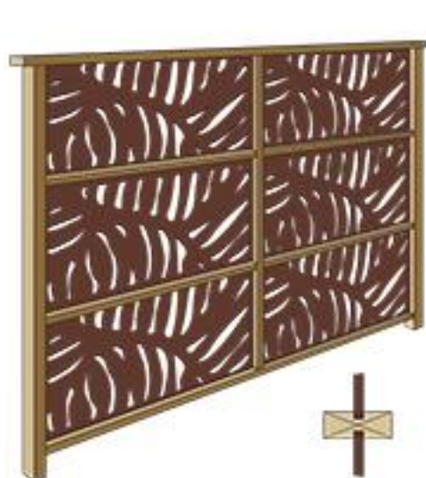
Window-Mount in Frame with Channel
