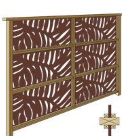
Window-Mount in Frame with Casing
