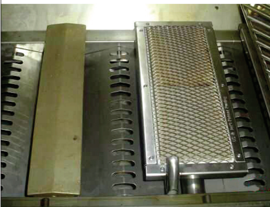
One Sear Zone burner installed
