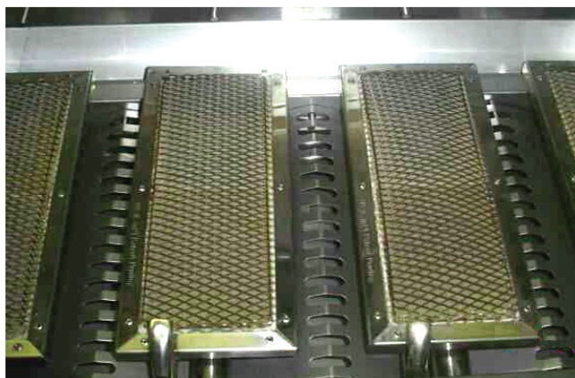
Multiple Sear Zone burners installed
