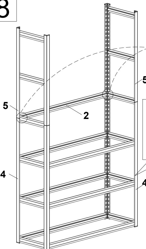
Snap part #2 into the hoist holes on the lower part of part #5 and the upper part of part #4 respectively. And tap them flat with a small hammer
