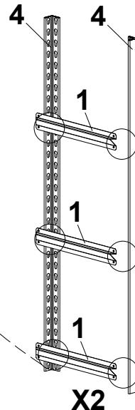
Install the other lower side frame in the same way, taking care to keep the installation height consistent
