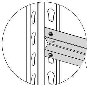
Using a small hammer, tap the flat side of part #1 (flat side up) so that the circular slot in part #1 is completely inside the hoist hole in part #4 (as shown)
