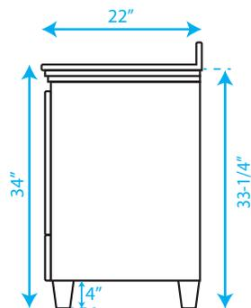
\*Note: Due to high probability of breakage-the backsplash comes in two pieces-cut from same piece. All measurements are  $\pm 1/4"$
