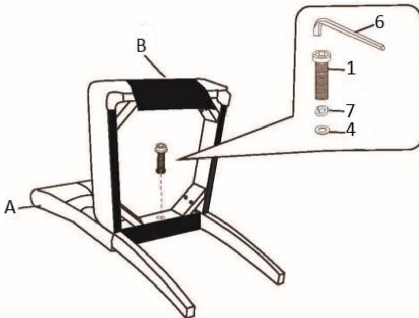
Align Seat (B) into pre-drilled holes on Chair Back (A).
