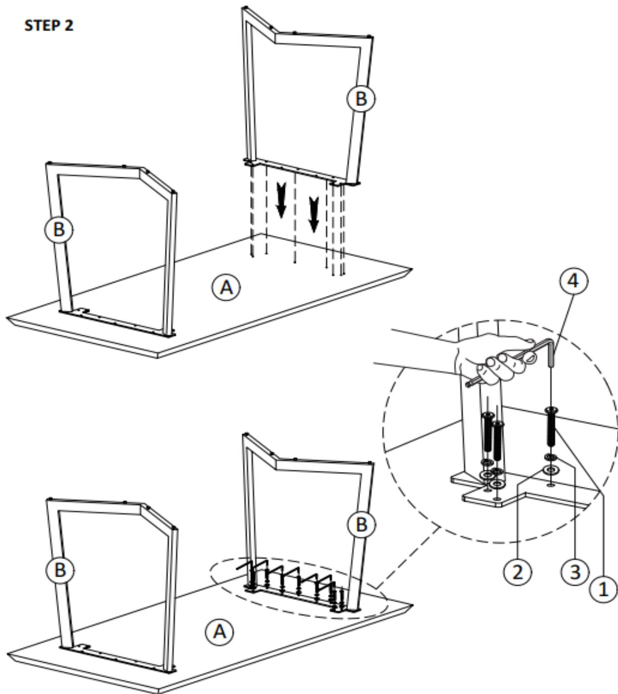
1. Repeat Step #1 to attach the second Leg (B) to Top (A).
