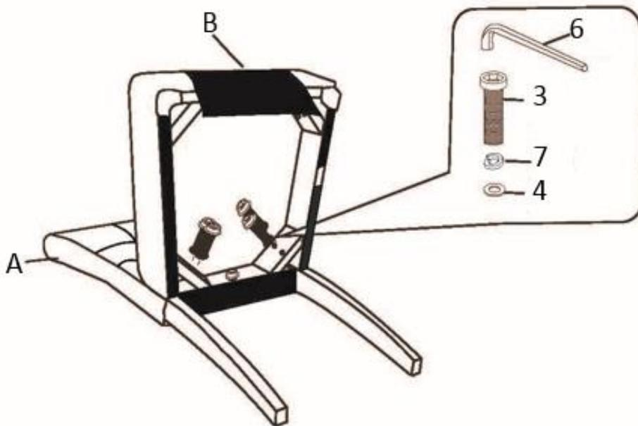
Attach Seat (B) to Chair Back (A) using Allen Key Screws (3) and four Washers each of (4) and (7).
