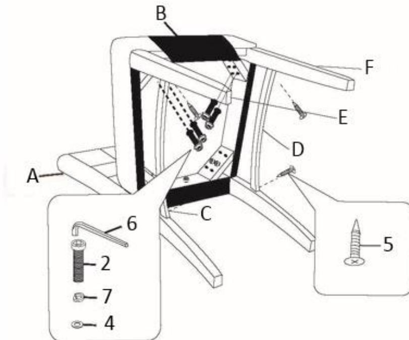
Attach Front Legs (E & F) using Allen Key Screws (2) and four Washers each of (4) and (7).
