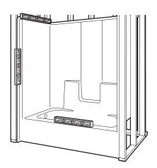
5. Pre-drill pilot holes. Fasten panel to framing at every stud and eight inches vertically through nailing flange.
