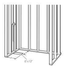
2. Place the unit into framing with drain fitting over and onto waste pipe with skirt firmly on the floor.
