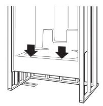
Assure waste pipe protrudes well into drain fitting.
