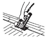
When installing wider plank wood floors (5" and wider) flooring movement due to seasonal changes may be reduced by utilizing both glue and the mechanical fasteners (nails/staples) specified. Do NOT use a moisture inhibiter with this application since glue assisted applications must have direct contact with the wood subfloor. Utilize a premium grade urethane construction glue (such as Liquid Nails® or Locktite® Urethane Wood to Wood Glue) and apply glue in a serpentine fashion to the subfloor.
