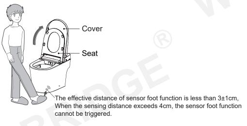
3. When the seat and cover are open, touch the sensing area with feet, close the seat and cover and then make the half flushing.
