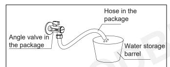
Open the angle valve and connect water inlet for 10s, once the water volume is above 0.66Gal (2.5L), the minimum water pressure of the product is ensured.
