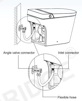
Connect the water inlet and angle valve of the toilet with the matching hose and tighten it
