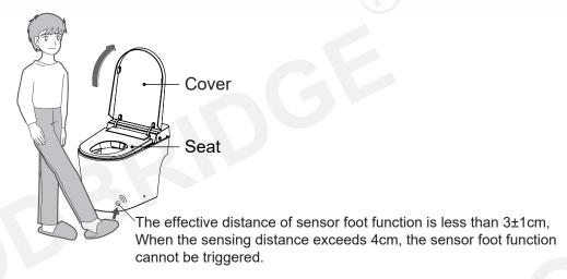
2. When the cover is open and seat closed, put the foot within the sensing area and then seat opens automatically.
