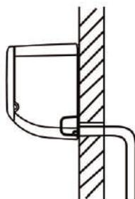
Make sure there are **NO** kinks or dents in the hose to ensure proper drainage.
