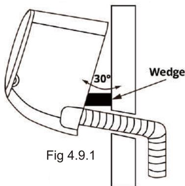
3. Connect drain hose and refrigerant piping (refer to **Refrigerant Piping Connection** section of this manual for instructions).
