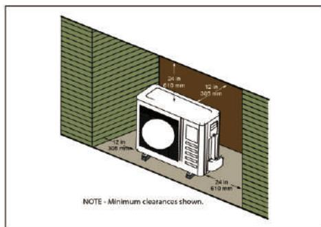
Fig 5.3.1. Unit installed in Alcove
