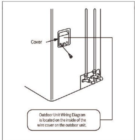
2. Unscrew the electrical wiring cover and remove it.
