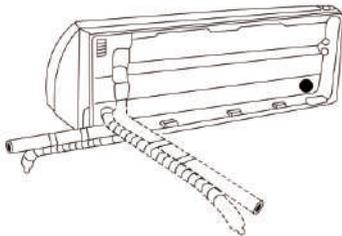
3. Use scissors to cut down the length of the insulating sleeve to reveal about 6 in (15 cm) of the refrigerant piping. This serves two purposes:
