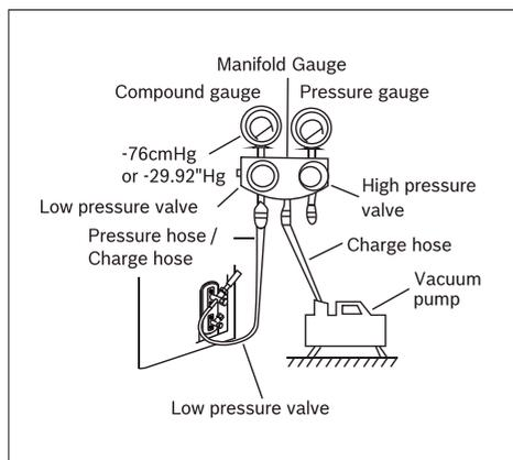
1. Connect the charge hose of the manifold gauge to service port on the outdoor unit's low pressure valve.
