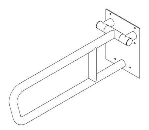
Locate the area with 2" solid wood in-wall backing on the desired mounting surface.
