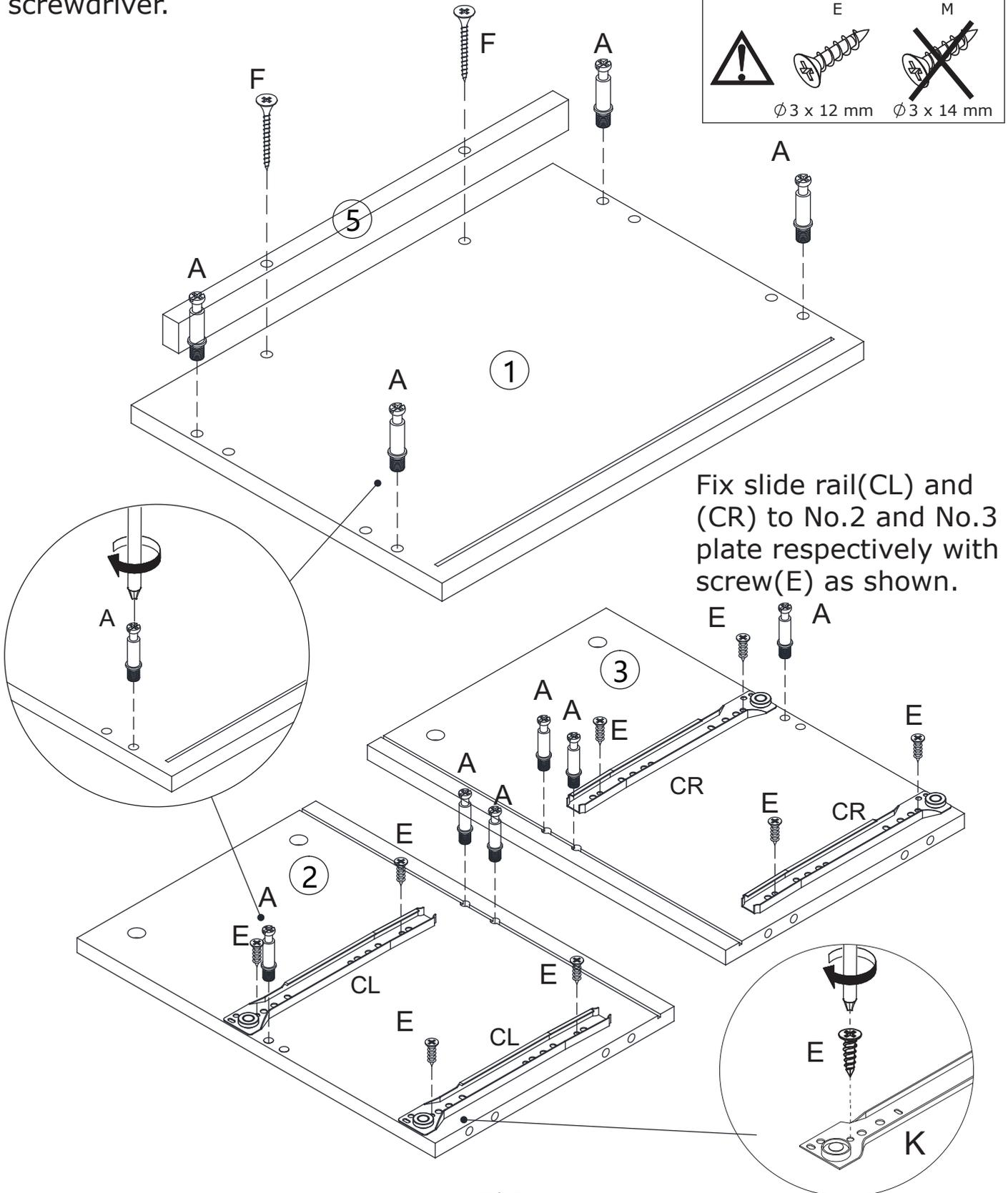
Fix slide rail(CL) and (CR) to No.2 and No.3 plate respectively with screw(E) as shown.
