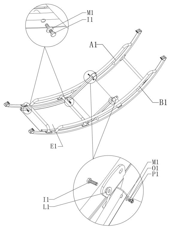
Friendly Tip: Please don't completely tighten the screws during assembly. After all the screws are assembled in place, tighten them together.
