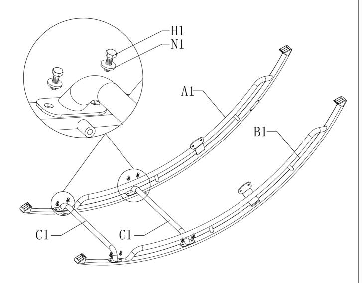
Friendly Tip: Please don't completely tighten the screws during assembly. After all the screws are assembled in place, tighten them together.
