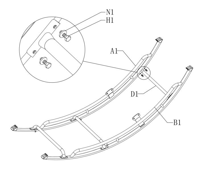
Friendly Tip: Please don't completely tighten the screws during assembly. After all the screws are assembled in place, tighten them together.
