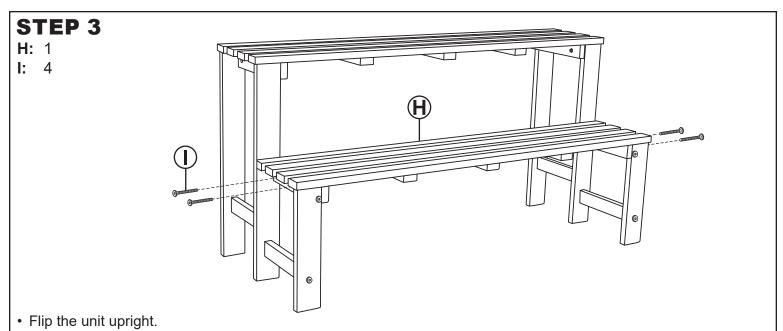
• Place Bottom Shelf (H) onto the lower level of the stand and secure it using four M6x45 Bolts (I). Tighten all bolts using Hex Key (M) after this step is complete.
