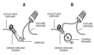
Connect wires according to the below chart
