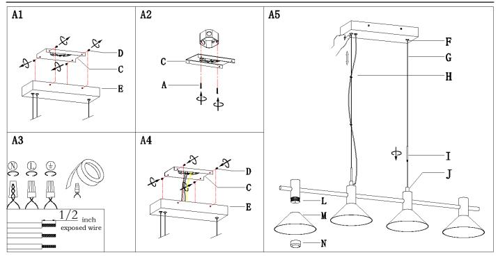
Step A1 » Unscrew screws (D) from mounting plate (C) and canopy (E).
