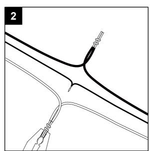
3. Attach wire nuts (CC). Tape wire nuts (CC) and wires together.
