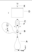
Step 1: Fasten Socket Assembly(B)onto Lamp body(A) Step 2: Squeeze the harp end (C) and inset into the sa Step 3: Install the bulb(F) on the socket. Step 4: Assemble the lampshade(D).
