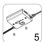
Insert the installation hole covers. Set all linked bars and pucks to the on position. Turn on the Dimmer Switch power button. Adjust the Dimming Slider to the desired
