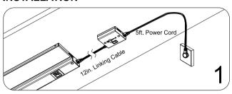
Place the product in the desired position. Ensure the 5ft. Power Cord (included with your bar or puck) can reach the outlet and that the 12in. Linking Cable (included with this package) can reach the nearest bar or puck. If your layout exceeds the distance between each fixture, swap the 12in. linking cable for longer
