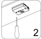
Pay attention to INPUT and OUTPUT direction. The Power Cord will connect to the INPUT side. Hold in place and to the IMPUT side. Hold in place and insert mounting screws. Provided screws are suitable for cabinet bottoms 3/8in. or thicker. Pre-drill a pilot hole for the screws using a 3mm or 1/8in. size drill bit if needed.
