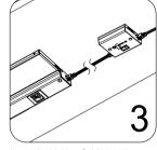
Insert the Linking Cable into the Dimmer Switch OUTPUT port and INPUT port of the adjacent bar or puck. DO NOT USE EXCEED 150W/1.25A LED OUTPUT.
