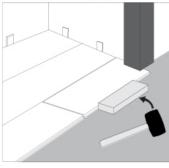
**Step 1:** Undercut door jamb to provide space to allow plank to slide freely. Tap long edge with hammer and tapping block to lock long edge.
