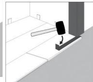
**Step 2:** Use hammer and pull bar to draw in and lock short end of plank.
