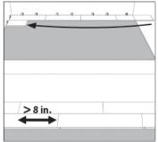
**Step 3:** Use the remaining plank from your cut piece to begin the next row (you will repeat this process throughout the installation). Note: It is recommended that you space end-joints by a minimum of 8 inches.
