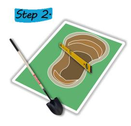
Using a digging shovel excavate the hole, starting with the deeper sections first.
