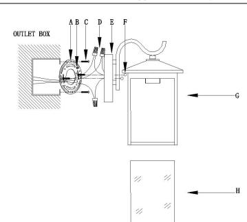
Unscrew the threaded balls (F) from the back plate then carefully Remove the mounting plate (A)
