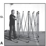
**Step 2:** With a partner, hold the top and bottom of the eave where it forms a diamond (Fig. B). Lift slightly and slowly walk backward until the frame is fully extended (Fig. C). Take care to avoid pinching your hands or fingers.
