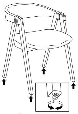
Turn clockwise or anti-clockwise to adjust leg leveller.
