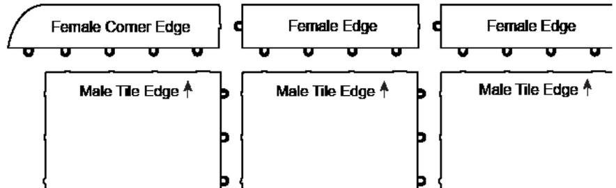
Alternatively, if your floor has an exposed side of female loops on the tiles, use a male edge kit to connect to them. See the illustration on the right.
