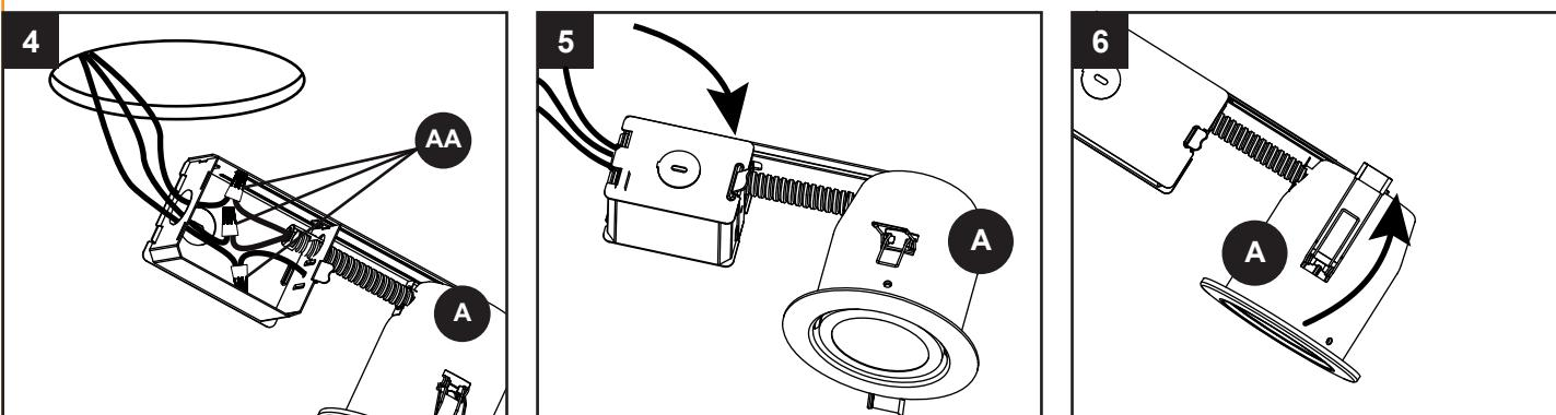
Connect the fixture wires to the supply wires – black to black, white to white, and green to copper/bare. Secure wires together with AA.
