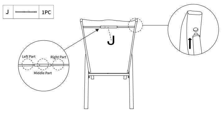
Step 7: Hold the middle part of the Part (J) and rotate the right part of it by clockwise until the seat back is fully extended.
