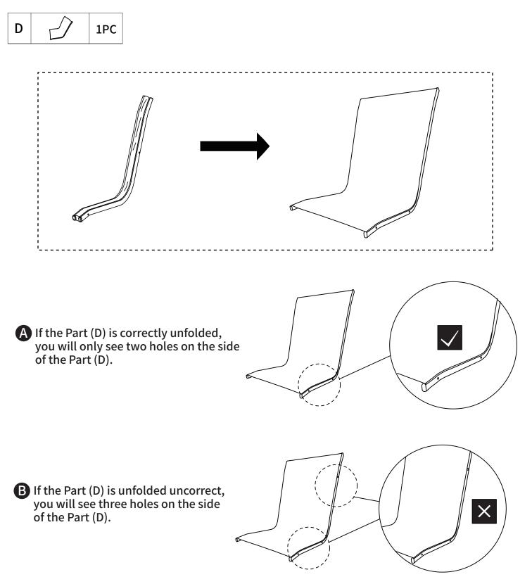
Step 4:Make sure you place the the part (D) on the chair frame at the correct direction. Align the holes of part (D) to the top holes of the support beam (C).
