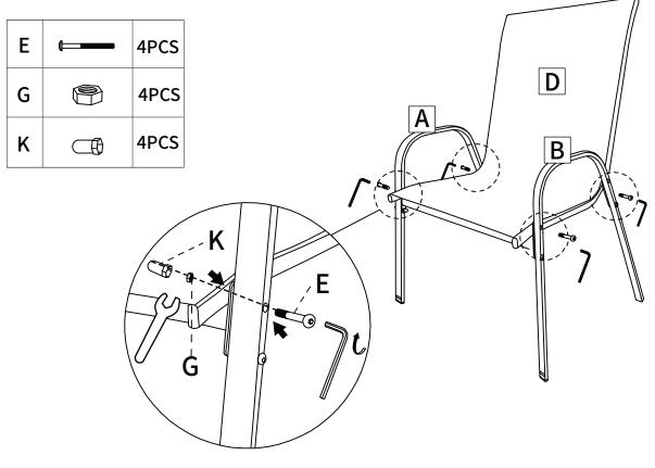
Step 6: First insert the left side of Part (J) into the Part (D). Then insert the right side of Part (J) into the Part (D).
