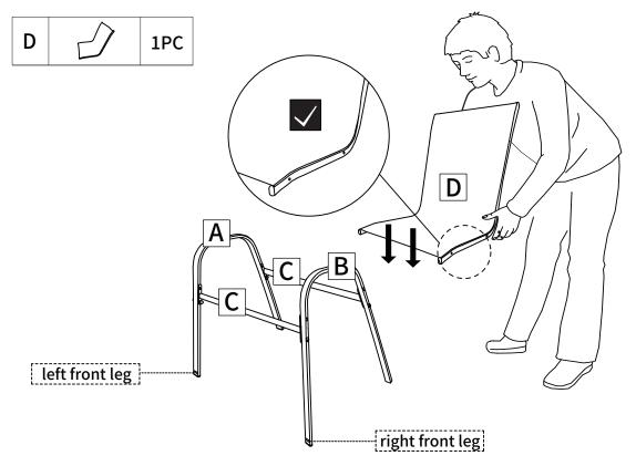
Step 5: Use screws (E) and nuts (G) and parts (K) to connect part (D) to the metal frame.After this step,you can tighten each screw.
