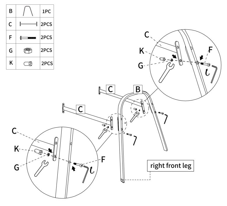
Step 2: After attch the right side of 2 support beams (C) to Right Leg (B), please attach the left side of 2 support beams (C) to Left Leg (A).Use screws (F), nuts (G), parts (K) to connect them.
