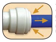
To disconnect, ensure that the system is depressurized, push the collet square against the fitting. With the collet held in this position the tube can be removed.
