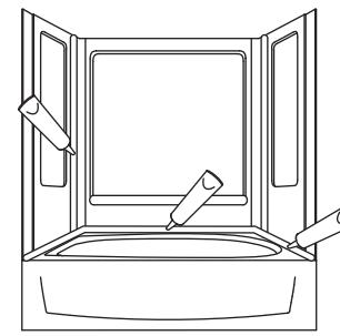
**22** After painting, apply 100% silicone sealant where the unit contacts the finished wall.
