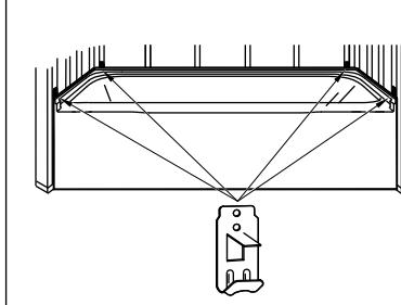
**8** Level the unit. Secure the metal support clips to the studs. Bend the tabs over the flange.
