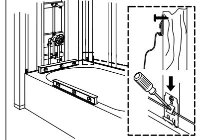
**9** Install plastic attachment clips at all remaining stud locations.
