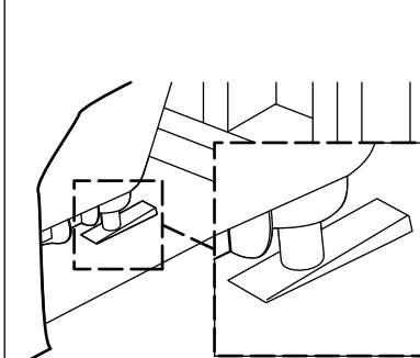
**11** Connect the bath drain to the drain pipe. Position a protective liner in the bath.
