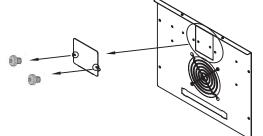
Remove the cover. The UV lamp is attached to the top of the back cover.
