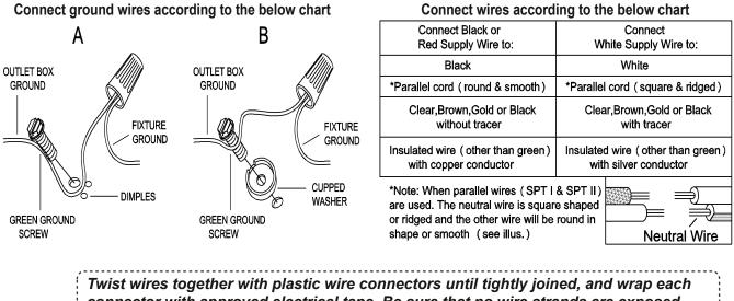
connector with approved electrical tape. Be sure that no wire strands are exposed and then carefully tuck all wires into the outlet box.
