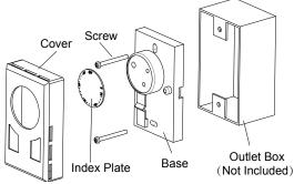
**Warning:** Turn OFF the power at the circuit breaker before installing. Installation should be performed by a qualified electrician. Refer to thermostat and heater load specifications before installation of the thermostat to see if it can handle the amp load. The maximum this thermostat can run is 7756 Watts at 277 Volts, 6720 Watts at 240 Volts, 5824 Watts at 208 Volts and 3360 Watts at 120 Volts.
