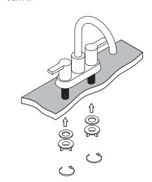
**4.** Connect the top of the hot and cold water pipes to the bottom of the hot and cold handles.
