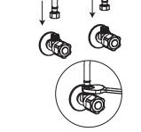
**3.** Place the rubber washer and plastic fixing nut in the bottom of the cold and hot water handles in turn.
