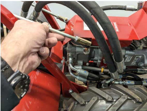
Install Wheel Control Rod Into Bracket on right side
