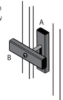
4. Turn Rail A to be level with Rail B at the desired height on railing.
