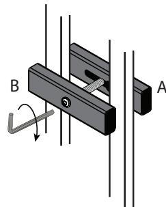
6. Connect Hold It Mate Accessory. If you'd like to position rail and accessory flush with the hand rail on your deck, simply loosen the sleeve nut with the accessory attached, slide them up and retighten.
