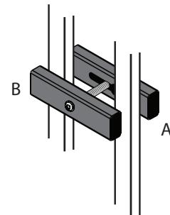
5. Once level, tighten sleeve nut with Allen wrench – do not over tighten – a snug fit will do. If releveling is needed, simply loosen the sleeve nut a little, adjust and repeat step.
