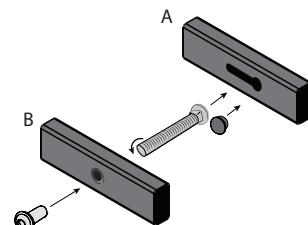
3. Hang Rail A horizontally so the bolt is up in the narrow end of the key hole slot, allowing it to fit through the decks spindles.
