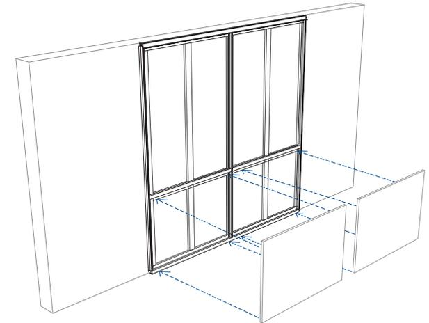
Position bottom wall panel between the chair rail and the bottom rail.
