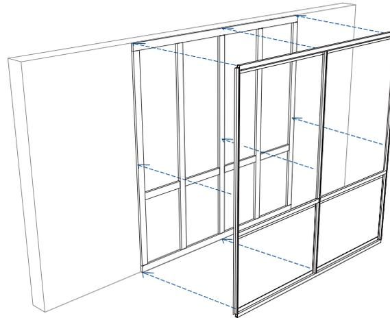
Install vinyl rail extrusions over the polystyrene strips using construction adhesive. Use 5/8" flat head screws to secure rails until adhesive cures.
